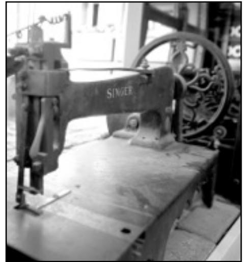
To repair shoes and boots, John uses the 1937 Singer sewing machine (below front) and two other Singer machines. He provides maintenance on the machines when necessary, saying one of the most common problems is that bobbin gears wear out.
