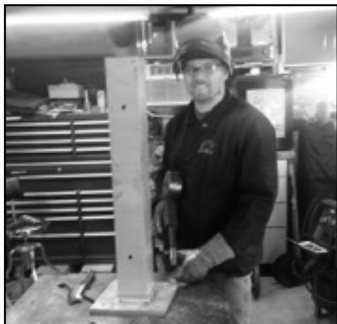
Jason Frey (J & F Fabrications) welded 21 brackets needed to support the newel posts.
